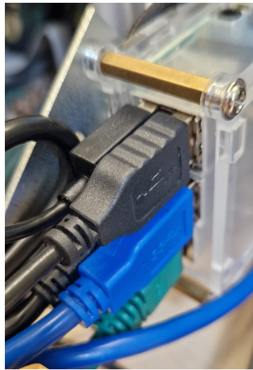
Figure 9: USB Connectors at the back of the Pi
